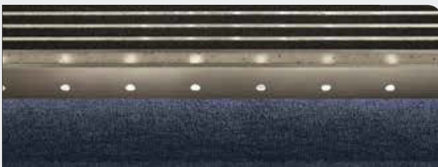
TOPDEC Series. 6mm visual holes at approximately 66mm centres allow the LED's to shine up through the off white visual front bar and through the visual holes at approximately 66mm centres in the riser of the nosing, whilst also fan lighting the riser and the tread below.
