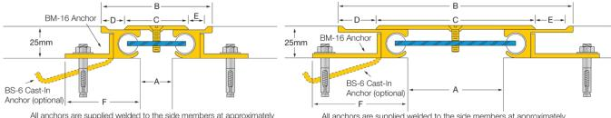
475mm centres. BM-16 anchors are supplied factory drilled with 10mm holes at approximately 475mm centres
