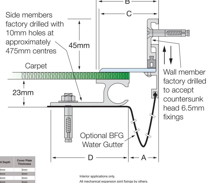
**Stainless Total Available Overall Depth** Steel Code Movement Movement ribbed deck DRCSL-25 +/-12mm 25mm 23mm +/-12mm 25mm 23mm DRCSL-75 75 +/-12mm 25mm 23mm 25mm +/-25mm 23mm 3mm DRCSL-150 | 150 | 177 | 175 | 68 +/-12mm 25mm 23mm 4mm
