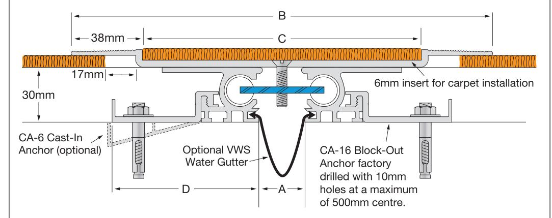
Aluminium Cover Plate Code Thickness Movement ribbed deck SCA-25 +38/-17mm 30mm 9mm SCA-50 +/-34mm 68mm 30mm 9mm SCA-75 75 +/-34mm 68mm 30mm 9mm SCA-100 +/-34mm 150 230 68mm 30mm 9mm
