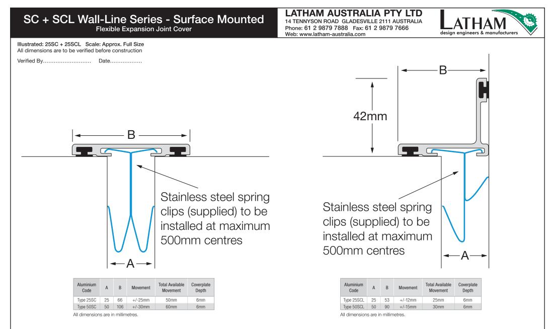
20 micron clear anodised aluninium finish (standard) or brass colour anodised aluminium finish (specify brass colour finish).
