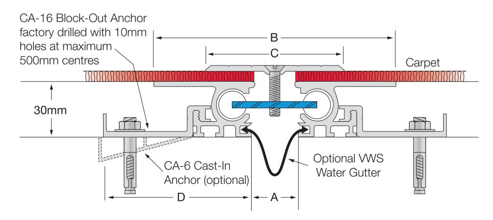
Aluminium Cover Plate Code Thickness Movement ribbed deck RCA-25 75 +25/-15mm 40mm 30mm 3mm RCA-50 +/-25mm 50mm 30mm 3mm RCA-75 75 125 +/-25mm 50mm 30mm 3mm RCA-100 100 208 +/-25mm 50mm 30mm 3mm
