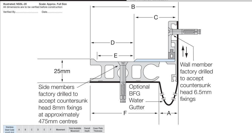
Wider joint widths available on request. All dimensions are in millimetres.
