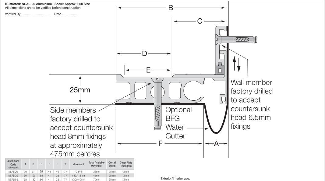
Wider joint widths available on request. All dimensions are in millimetres.
