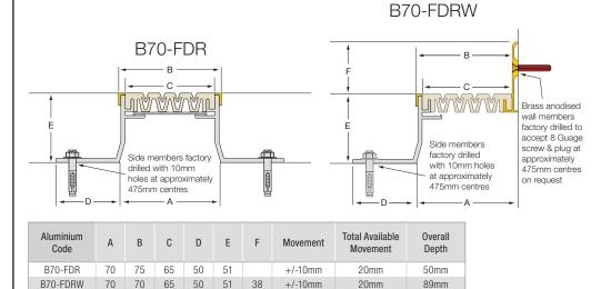
$\gamma$ Side members factory Side members factor drilled with 10mm drilled with 10mm holes at approximately holes at approximately 475mm centres 475mm centres on request Aluminium Total Available Overall Movement R C D F Code Movement Depth 50 31 +/-10mm 20mm 31mm B70-FDR (30) 70 75 65 65 B70-FDRW (30) 70 70 50 31 38 +/-10mm 20mm 69mm
